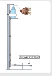
Press paddle by foot, maintaining a safe distance between hand and sanitizer bottle.
