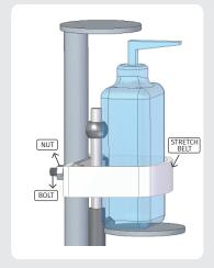
Once gap is set, place the bottle and tie with stretchable belt.
