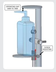
Set the Gap (5-7mm) by adjusting to bolt as shown.
